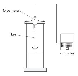
The apparatus shows a force meter that pulls on the attached fibre. The force needed to break the fibre is recorded on the computer.
